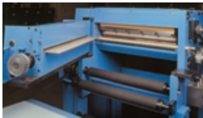
Swing Away Assembly for Easy Access to Bed Knife
